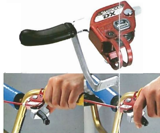
One Tap Gear Change—High to Low. One Tap Gear Change—Low to High.
