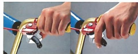
One Tap Gear Change—High to Low. One Tap Gear Change—Low to High.
